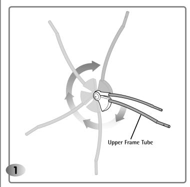
• Rotate the upper frame tube until it "snaps" into an upright position, as shown.
